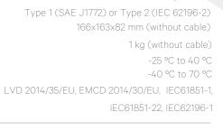
7,4 kW (1P) / 22 kW (3P)<sup>(2)</sup> 110/230V AC ± 10% (1P) / 400V AC ± 10% (3P)<sup>(2)</sup> 32 A, 5x6 mm² cable Charging current configurable from 6 A to 32 A 50 Hz / 60 Hz IP54 / IK08 CAT III AC 30 mA / DC 6 mA External RCCB<sup>(3)</sup> required
